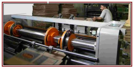
Double wall corrugators (Japan) with controlled temperature and moisture during production, working capacity of 30 meters in one minute.
